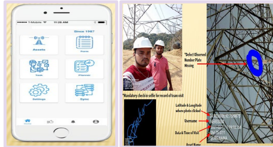
Application-based inspection tool for proactive approach to maintenance
